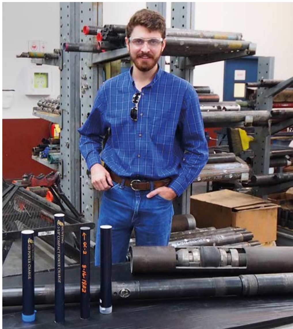
Pictured right: Engineer Ty Stovall presents the Power Charge family which are used in Setting Tools to set a plug before perforating and fracking a well.
