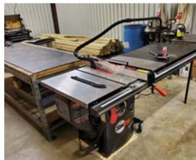
When skin contacts the blade, the signal changes because the human body is conductive. The change to the signal activates the safety system
