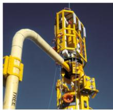
FAMs create an universal port in the 'Jumper' flowline on the seabed, enabling the use of standard Xmas Trees and Manifolds. With the FAM providing LoF flexibility within the system design, it enables Smart Standardisation to maximise the functionality of standard subsea hardware and accelerate field development.
