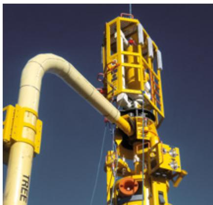
FAMs create an universal port in the 'Jumper' flowline on the seabed, enabling the use of standard Xmas Trees and Manifolds. With the FAM providing LoF flexibility within the system design, it enables Smart Standardisation to maximise the functionality of standard subsea hardware and accelerate field development.
