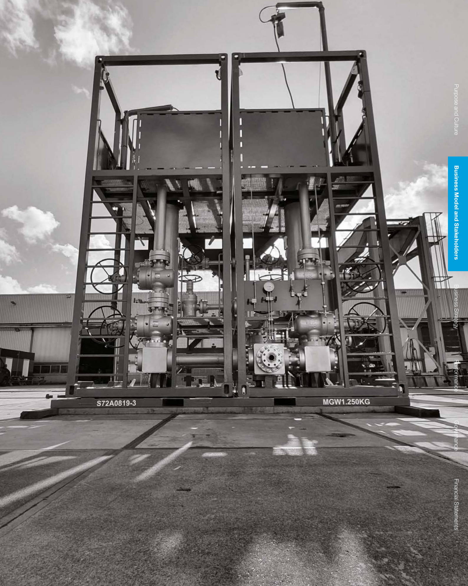
A Dual Pot Sand Filter manufactured by the Well Testing business in the Netherlands.
