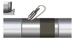
Arming Instructions: The HT73 has a directional output. The main load end of detonator must face the direction of the explosive train toward the shaped charges.
