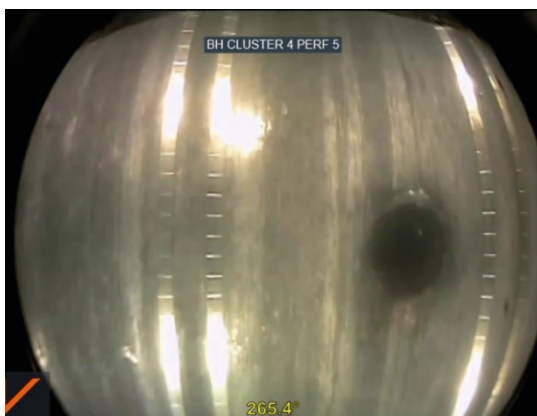
Figure 1 – EV camera perforation
